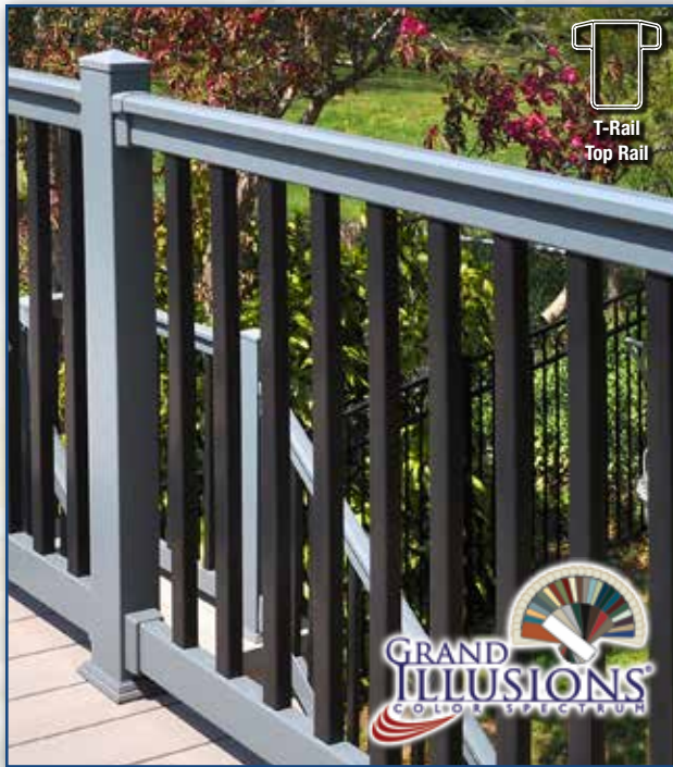
VRT6/8-3 Traditional Picket 1.5" x 1.5", T-Rail Top and 2" x 3.5" Bottom Rail - Shown in Millennium Gray (E104) and Black (L105)
